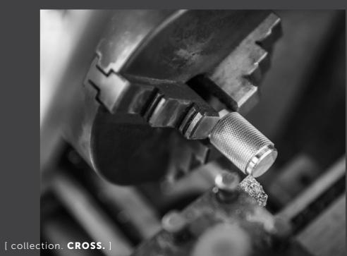
Our signature cross-knurl pattern is diamond-cut into 20mm diameter solid bar and inspired by machinery. Industrial in look and scale this knurl feels amazing under touch. The cross-knurl is accompanied by our signature solid metal coin screws.
